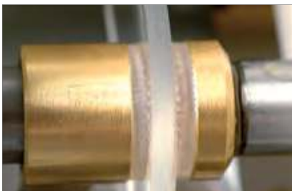
Soft silicone chuck pads ensure a secure grip of the lenses and an even distribution of pressure when clamping them
